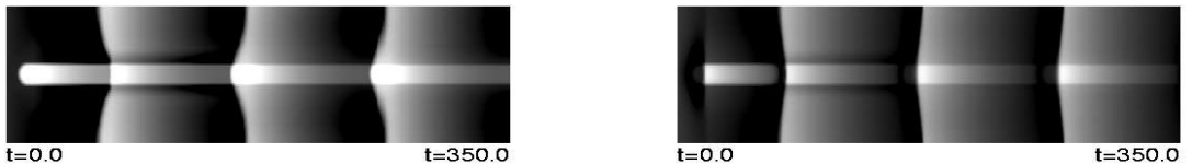
Figure 5: 1-D simulation with non-Fickian diffusion showing the development of reaction fronts as stable response. A permanent perturbation via modification of the PDE parameters in the center was used to mimic the effect of surface defects. Initial conditions (ic's) are set homogeneously. Same parameters as in Figure 2 were used. Site blocking constants set to (9). PBC applied. (top) \theta_{1\times 1} , with z_{max} = 0.70 and z_{min} = 0.20 ML, (bottom) \theta_{\text{NH}_3}^{1\times 1} , with z_{max} = 0.20 and z_{min} = 0.02 ML. Note the higher velocity of this second front in agreement with PEEM experiments.
