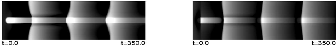
Figure 5: 1-D simulation with non-Fickian diffusion showing the development of reaction fronts as stable response. A permanent perturbation via modification of the PDE parameters in the center was used to mimic the effect of surface defects. Initial conditions (ic's) are set homogeneously. Same parameters as in Figure 2 were used. Site blocking constants set to (9). PBC applied. (top) \theta_{1\times 1} , with z_{max} = 0.70 and z_{min} = 0.20 ML, (bottom) \theta_{\text{NH}_3}^{1\times 1} , with z_{max} = 0.20 and z_{min} = 0.02 ML. Note the higher velocity of this second front in agreement with PEEM experiments.
